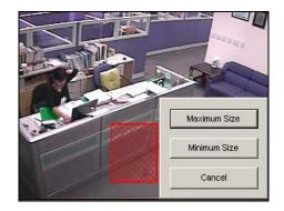
Figure 1-64 Defining the min. and max. detection size
