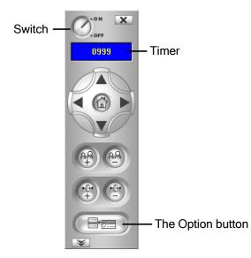
Figure 6-34 PTZ control panel
